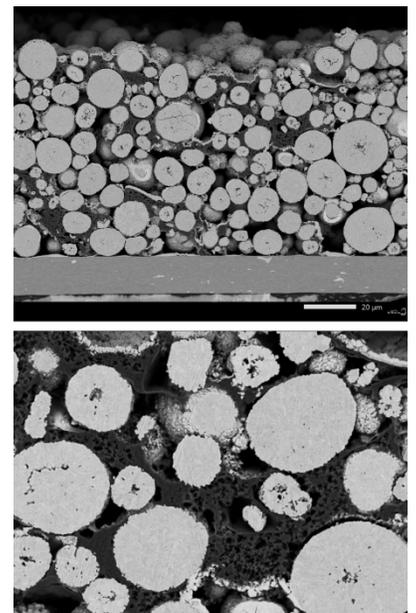
Fig. 2. Backscatter image of LIB cross-section prepared with JEOL CP polisher.
