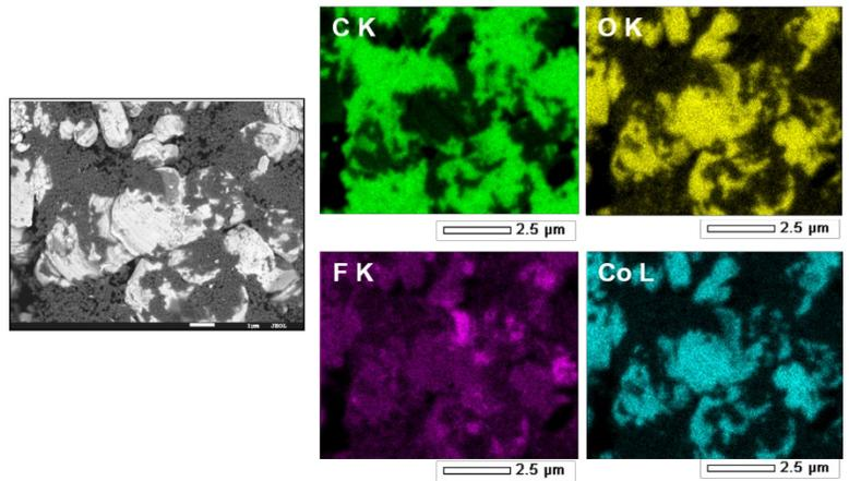
Fig. 1. EDS map of LiB cathode at 1.2kV, 6nA, 10kX. The map shows distribution of C, F, Co and O. Taken with JEOL FESEM.
