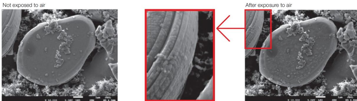
Fig. 3:  $\text{LiCoO}_2$  particles in positive electrode before and after air exposure. Clearly, air exposure introduces various artifacts affiliated with specimen reactivity with atmospheric oxygen.
