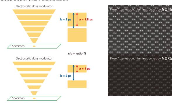
Dose attenuation by pulsed illumination with Frequency of 500 kHz (2  $\mu$ s) in a high resolution STEM at 300 kV using Si [110] in the condition of pixel dwell time with 19  $\mu$ s/pixel (1024  $\times$  1024 pixels), by changing duration ratio from 90% to 50% during acquisition of one STEM image in 20 s.
