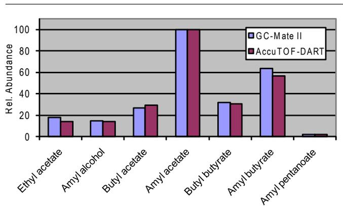
Figure 2. Comparison of relative abundances observed for compound using GC-MS and DART-MS analysis.
