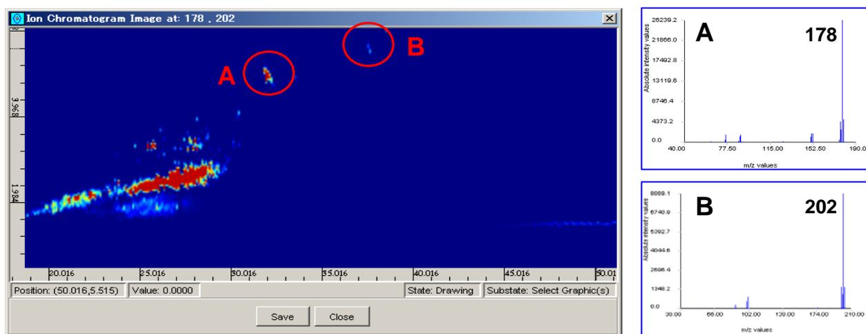
*Fig.2 : GC×GC mass chromatogram of  $m/z$  178 and 202 for polycyclic aromatic hydrocarbons and the corresponding mass spectra for the tri- and tetra-cyclic aromatic hydrocarbons.*
