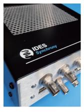
The Electrostatic Dose Modulator (EDM) is a fast beam blanking system with a pre-sample electrostatic deflector, including electronics and software control. With EDM, the 100,000x improvement in blanking speed immediately improves the clarity of data taken at fast exposure times. EDM can also attenuate electron illumination without affecting imaging conditions, giving TEM and STEM users exceptional control over the dose on their samples.
